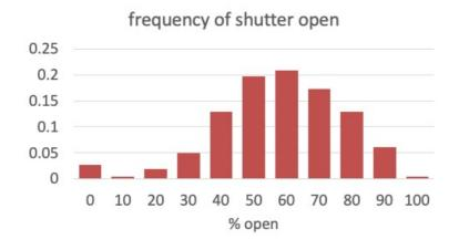
In any case the shutter open, summing all the programs and filler is typical for an imaging camera, and its is visualised in the above histogram.
